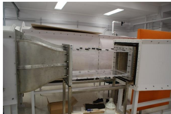
Figure 1: Wind tunnel contraction and test section containing a 4mm spray bar
