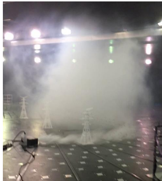
Figure 2: Full aero-elastic transmission line model under a simulated tornado conducted in WindEEE research institute
