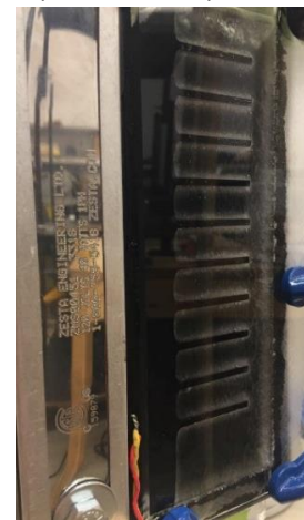
Figure 2: A photo of an experimental setup being developed to characterize heat transfer to PCM from fins
