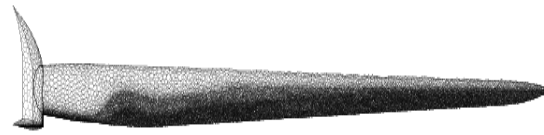
Figure 1: CFD mesh of a wind turbine blade
